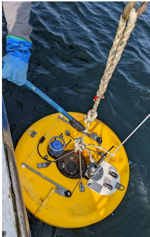
Figure 3-5: Sacrificial rope sling being cut with a knife during deployment of an OBS.
