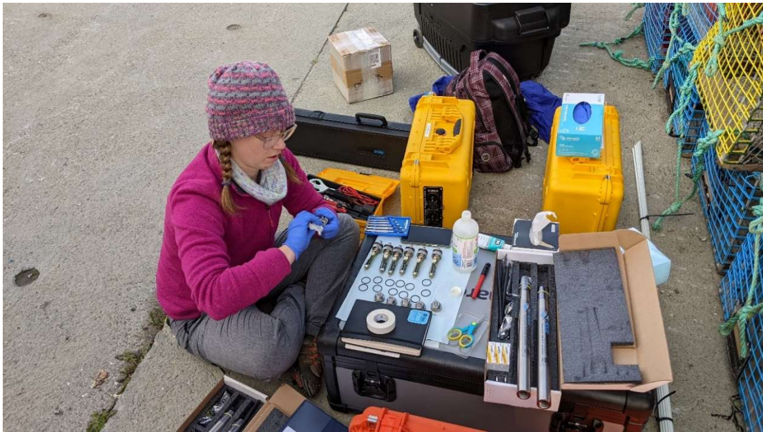
Figure 2-1: Assembling XMB-11k VHF radio beacons on the pier prior to departure.
