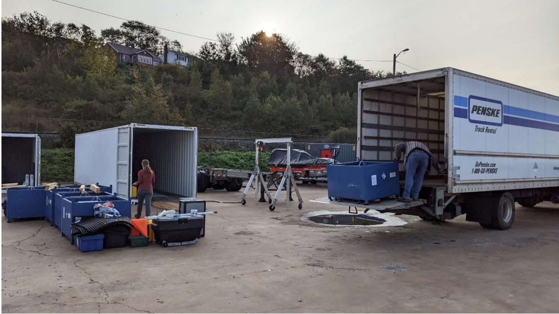
Figure 3-1: Loading Aquarius OBS in stillage boxes into 26-foot box truck using lift gate and pallet jack.
