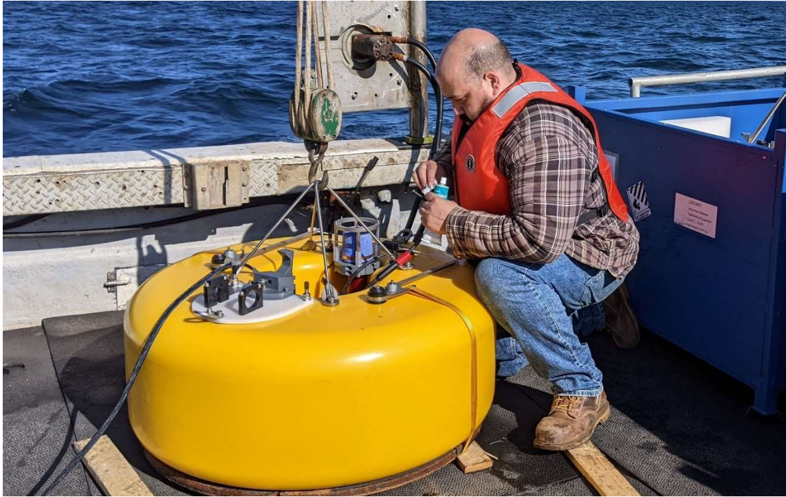
Figure 2-3: Cleaning and greasing Subconn electrical connectors on the boat's deck while underway.
