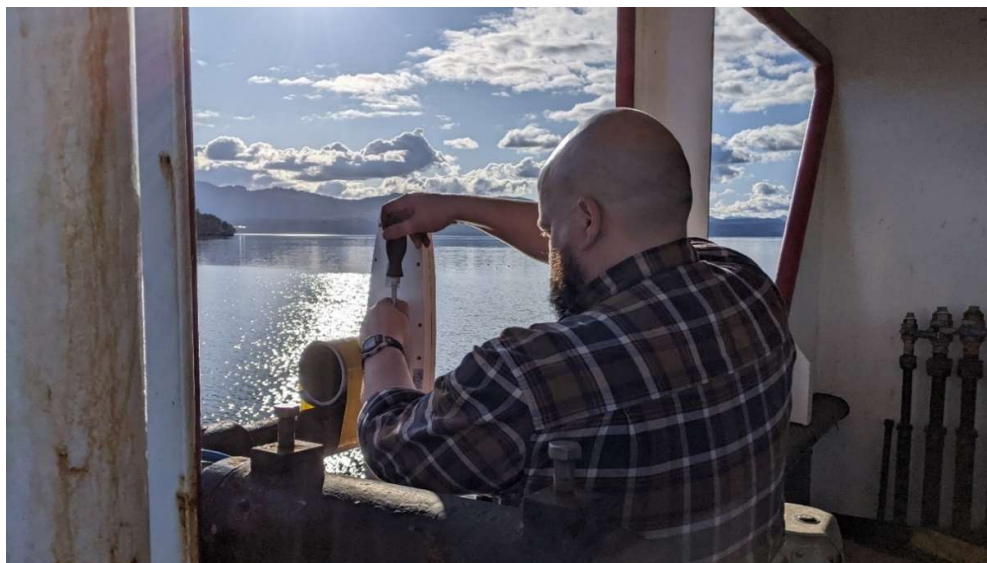
Figure 3-6 - Mounting of GPS receiver on top end of USBL pole. This configuration, which had been used by previous groups, gave poor GPS reception. GPS input from the ship's navigation system was substituted later in the cruise.
