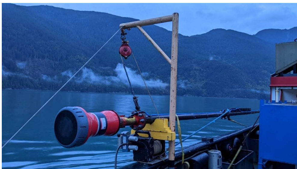
Figure A-2: LMF GyroUSBL transceiver mounted on side-along pole of CCGS John P Tully (stowed/transit position).
