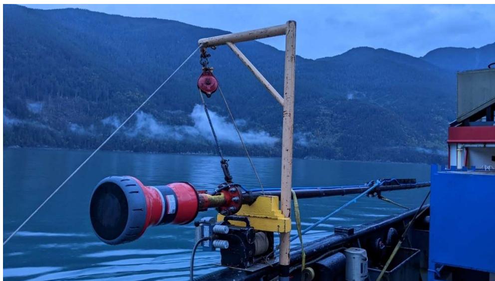
Figure 3-3 - Sonardyne Ranger 2 GyroUSBL mounted on port side pole of CCGS John P. Tully.
