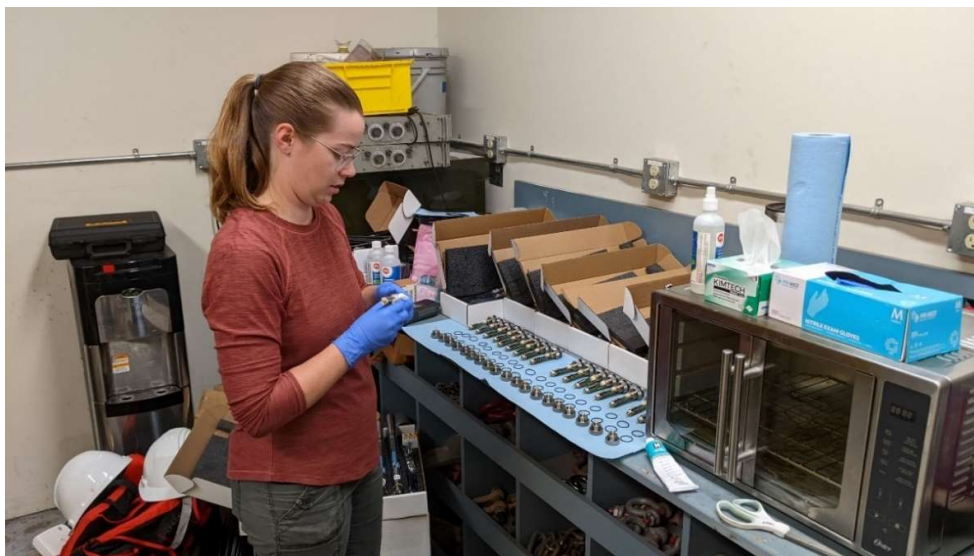
Figure 2-1 - Katie Bosman cleaning O-rings on the Xeos recovery devices in the IOS hangar workshop.
