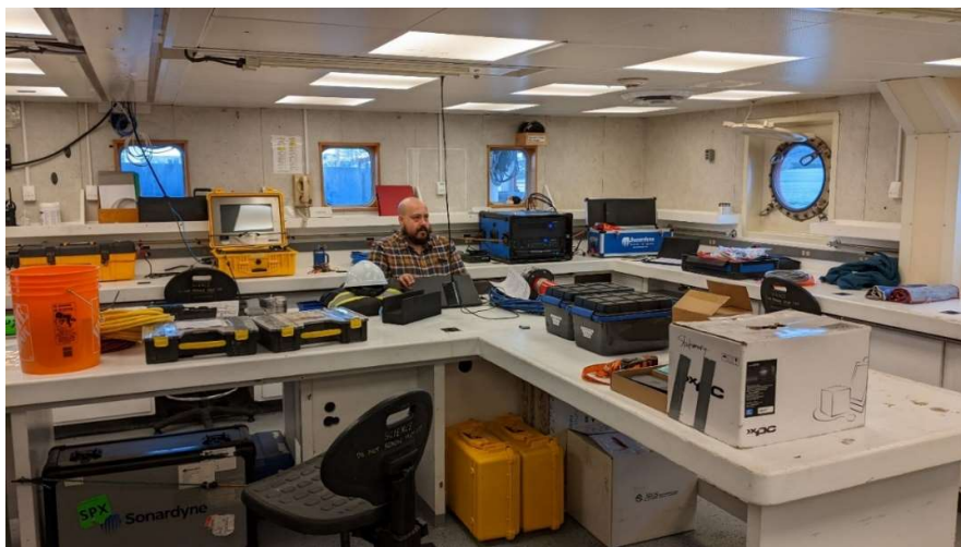
Figure 3-7 - Laboratory setup onboard Tully. The large blue box in the back right hand corner is the USBL computer running Ranger 2. The yellow Pelican case computer left of center is an Aquarius Deck Unit, used for programming the OBS via a cable run through a conduit over the window.
