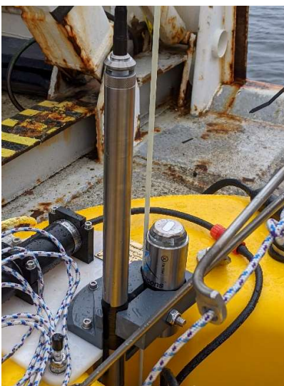
Figure A-1: Recovery devices mounted on OBS. XMB-11k VHF beacon on left, Apollo Mono GPS/LED/Iridium beacon on right.
