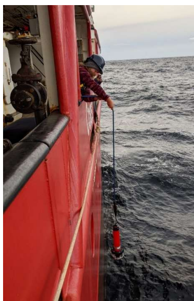
Figure 3-8 - Sonardyne omni-directional dunker being deployed over the side of the ship from the wet lab.
